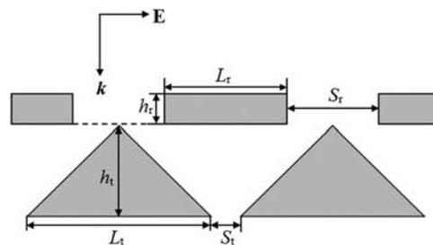
Fig. 1. The proposed hybrid gratings and their structural parameters.
