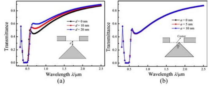
Fig. 6. Transmission spectra of the hybrid gratings with different vertical and horizontal relative displacements: (a) different vertical relative displacements; (b) different horizontal relative displacements.
