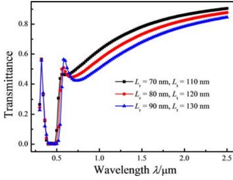
Fig. 5. Transmission spectra of the hybrid gratings with different  $L_r$  and  $L_t$  which are varied synchronously with fixed  $S_r = 60$  nm and  $S_t = 20$  nm.
