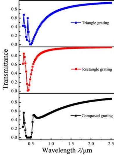
Fig. 2. Transmission spectra of the hybrid grating, the rectangle grating, and triangle grating.
