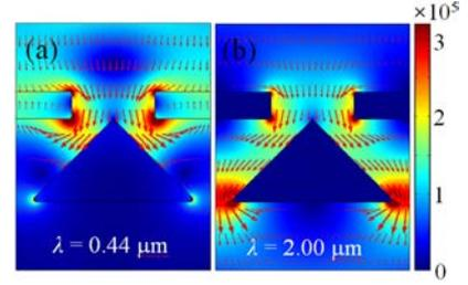
Fig. 3. Distribution of the electric fields and energy flows at different wavelengths: (a)  $\lambda = 0.44$   $\mu\text{m}$ ; (b)  $\lambda = 2.00$   $\mu\text{m}$ .
