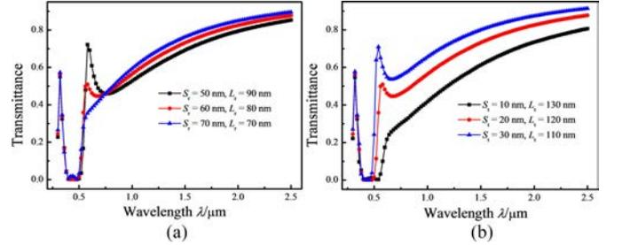
Fig. 4. Transmission spectra of the hybrid gratings with different separations: (a) different  $S_r$ ; (b) different  $S_t$ .
